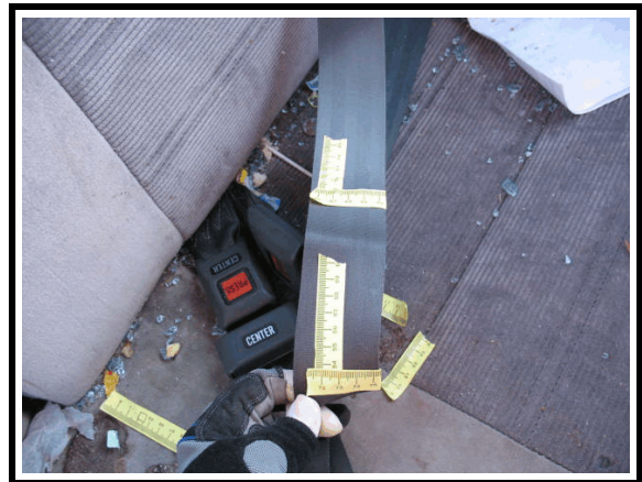
Figure 21. Scuffs and indentation on LR seat belt
