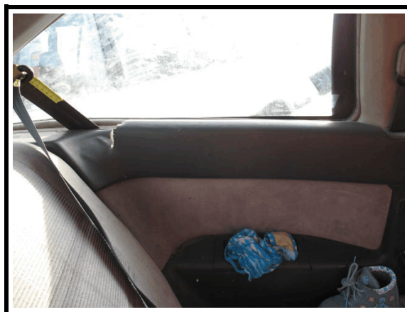
Figure 19. Damage/Intrusion to left rear side panel
