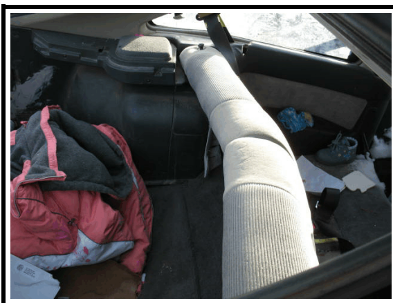
Figure 18. Second row seat back deformed from impact of rear cargo
