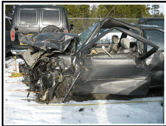
Figure 2. LF damage - 1986 Honda Accord
