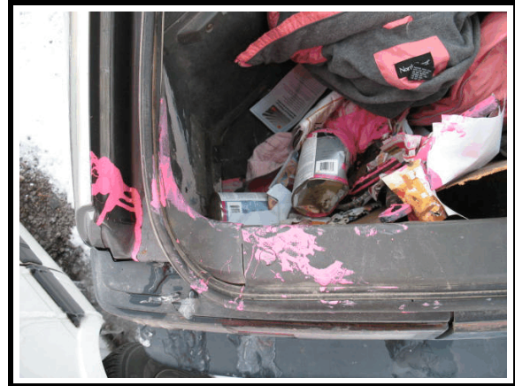
Figure 16. Hatchback opened during crash - paint found outside of rear cargo area
