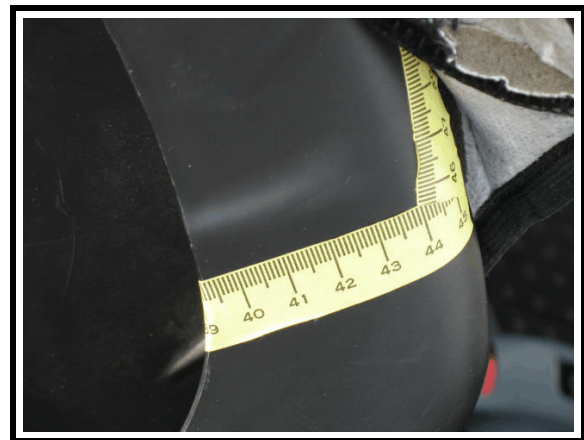
Figure 27. Close-up – stress mark on right side of booster seat
