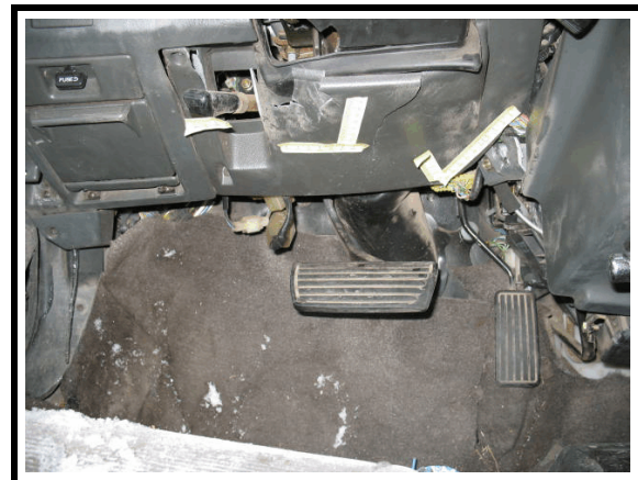
Figure 31. Occupant contacts to steering column and left instrument panel
