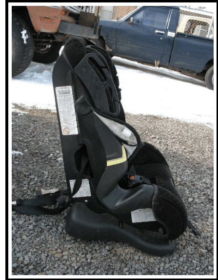
Figure 26. Stress mark on right side of CSS (highlighted with yellow tape)
