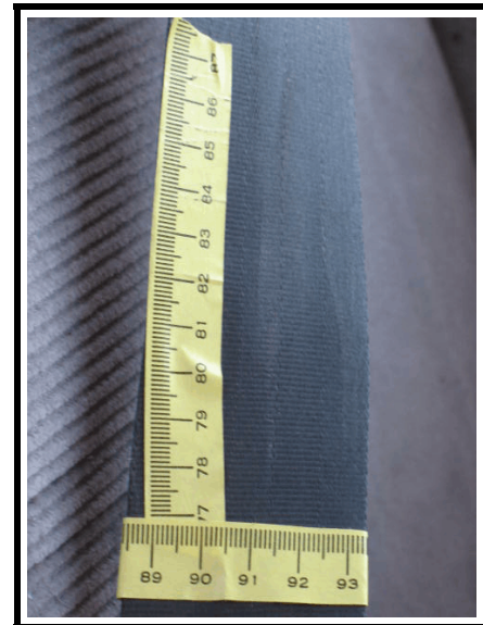
Figure 33. Evidence of loading to the second row left seatbelt
