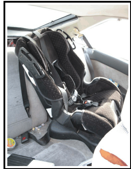
Figure 22. Dorel Alpha Omega child safety seat as found in vehicle
