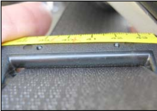
Figure 7. Left rear latch plate frictional abrasions.
