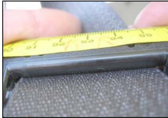
Figure 8. Frictional abrasions on the rear right latch plate.
