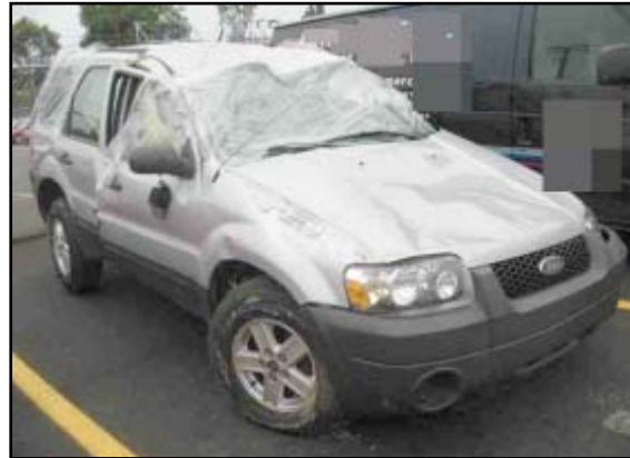
Figure 1. Rollover damage to the 2007 Ford Escape.
