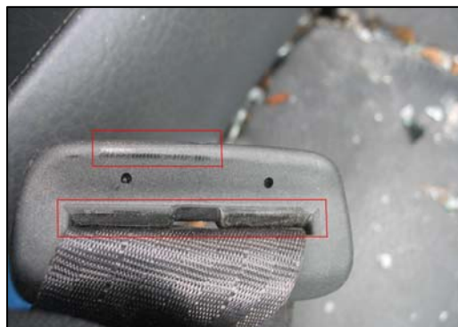
Figure 12 - Loading evidence on RF latch plate housing.
