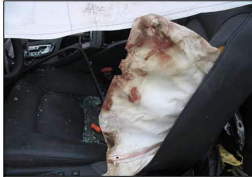
Figure 15 - Deployed driver's seat mounted side air bag.
