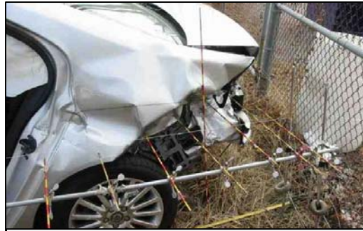
Figure 8 - Damage to left quarter panel from Honda CRX.
