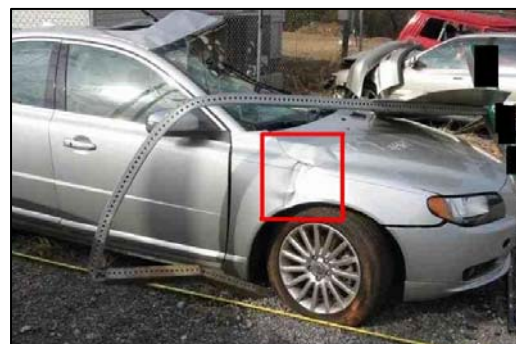
Figure 7 - Damage to right side of Volvo from signpost.
