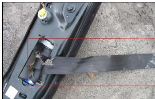
Figure 11 - Damaged B-pillar and retractor pretensioner.
