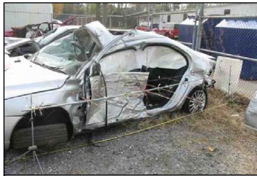
Figure 9 - Damage to left side of Volvo from tree impact.
