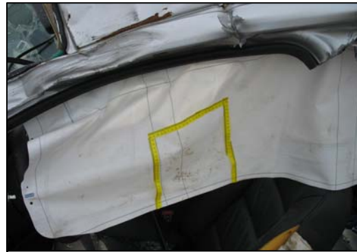
Figure 14 - Transfer evidence on outboard aspect of the IC air bag.
