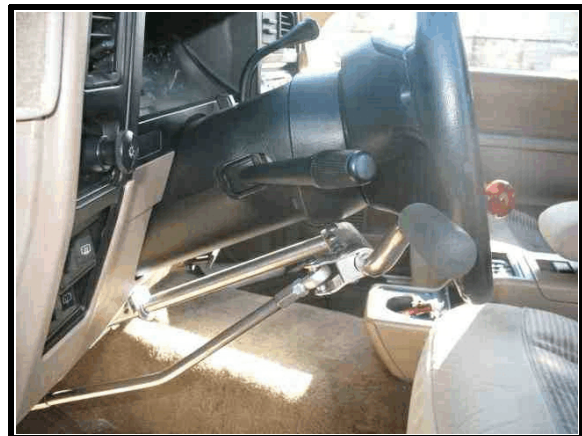
Figure 4. Side view of hand control installation
