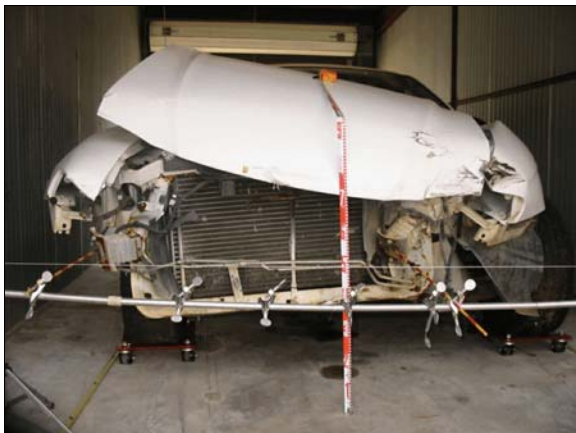
Figure 4: Damage to front of case vehicle from impact with the Five Hundred, vertical scale in tenths of meter
