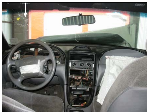
Figure 7: Overview of case vehicle's front seat area, arrow shows "star burst" type fracture to windshield from driver's head contact
