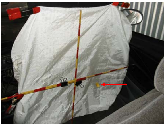
Figure 10: Case vehicle's front right passenger air bag, arrow shows location of small reddish/brown spot
