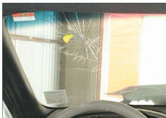
Figure 13: “Starburst” type fracture to the windshield due to contact by unrestrained driver’s head
