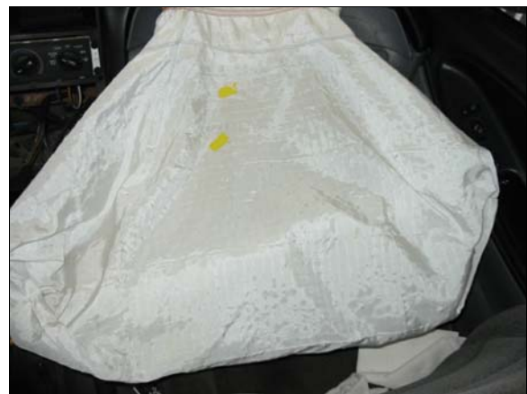
Figure 11: Top of case vehicle's front right passenger air bag, yellow tape shows location of small yellow spots
