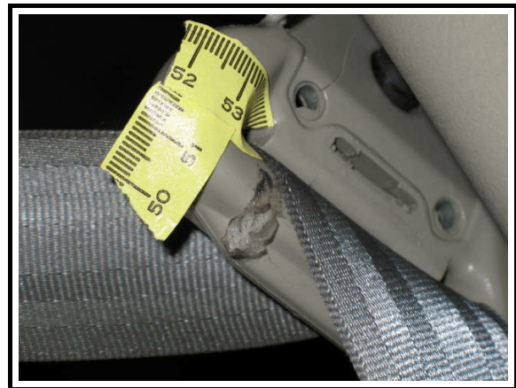
Figure 23. Driver's seat belt, frayed webbing fibers on D-ring
