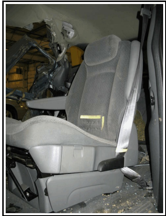
Figure 10. Second row left seat belt found routed through seat back adjustment lever
