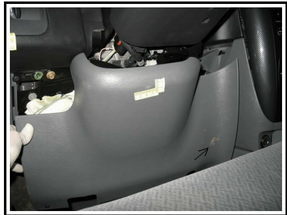
Figure 9. Scuffs to lower left instrument panel/knee bolster cover
