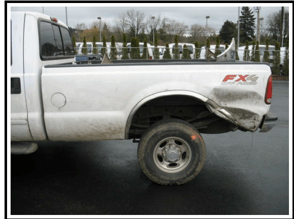
Figure 22. Left rear intra-unit contact damage
