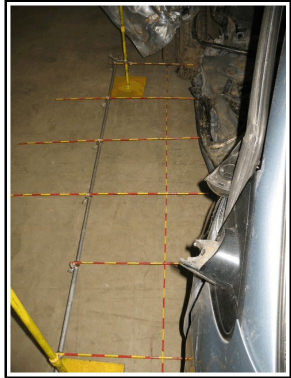
Figure 6. Right side crush profile (sill level)
