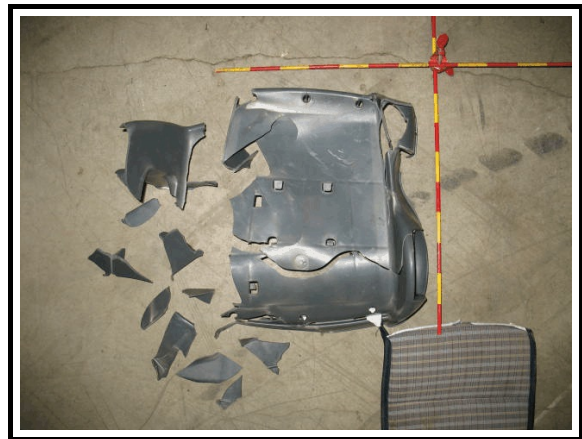
Figure 19. Cosco Dorel booster seat, showing damage
