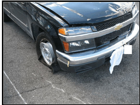
Figure 2. Front right bumper corner damage
