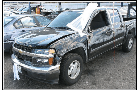
Figure 1. 2006 Chevrolet S10, left side rollover damage
