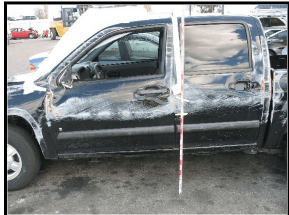
Figure 7. Overview of left side rollover damage
