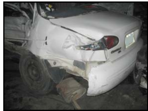
Figure 10: Left rear quarterpanel damage.
