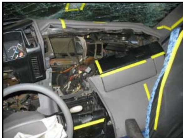
Figure 13: Center instrument panel contacts.
