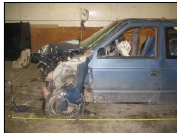
Figure 8: Forward left side damage.
