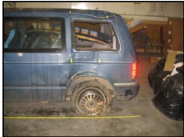
Figure 7: Left rear tree impact damage.
