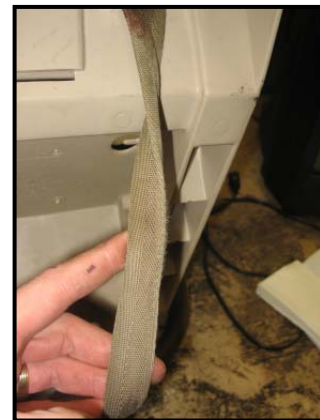
Figure 15: View of the buckled and deformed T-shield.
