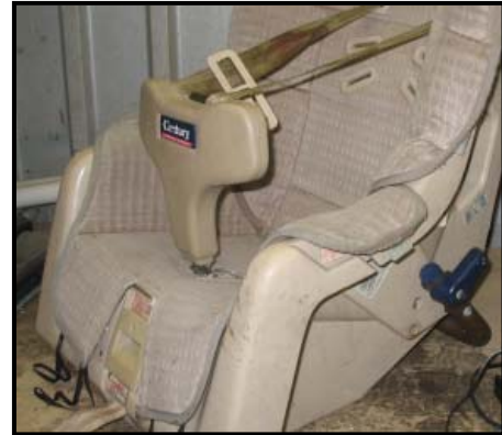
Figure 15: View of the buckled and deformed T-shield.
