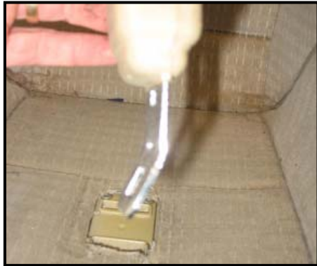
Figure 16: Close-up view of the deformed latch plate.
