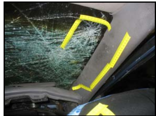
Figure 12: Right windshield fracture and A-pillar contact.
