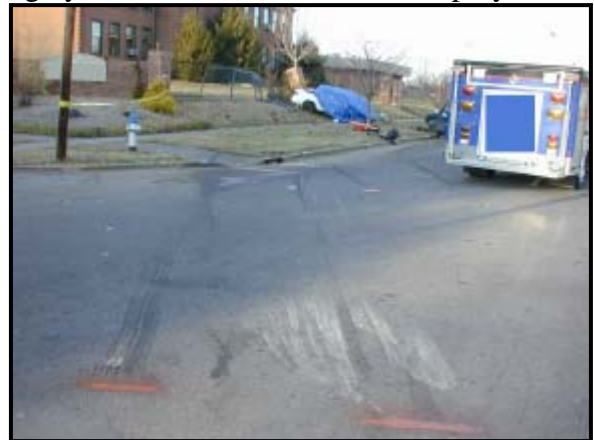
Figure 5: Point of impact and post-crash vehicle trajectories.
