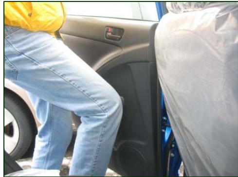
Figure 8. SCI investigator activating power window switch with his right knee.
