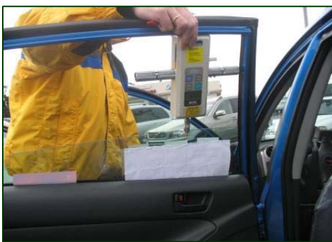
Figure 9. Force gauge positioned in the left rear window of the exemplar vehicle.
