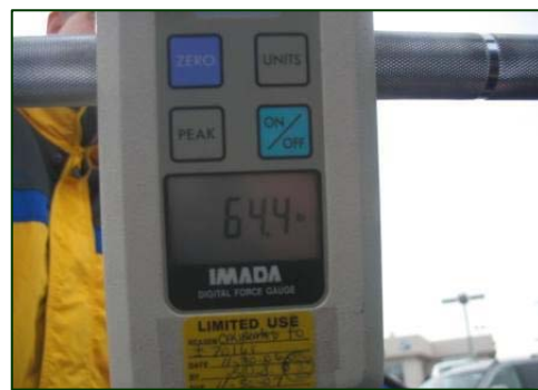
Figure 10. Highest reading exerted by the power window with battery power only.
