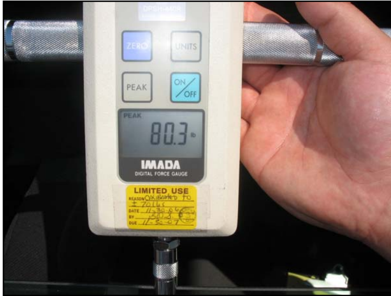
Figure 11. Peak closure force with the engine running.
