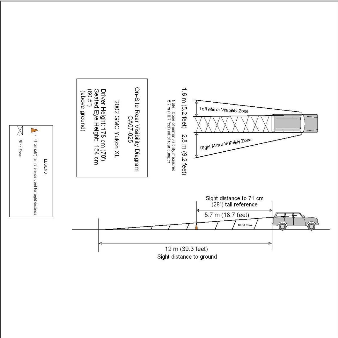
**Figure 15: Rear Visibility Diagram**
