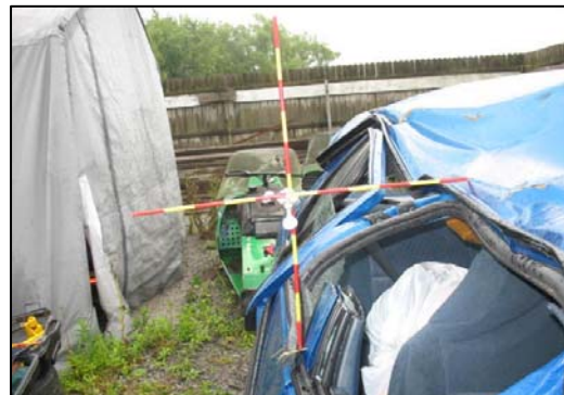
Figure 7 - Right side gauge placement on the Cavalier.
