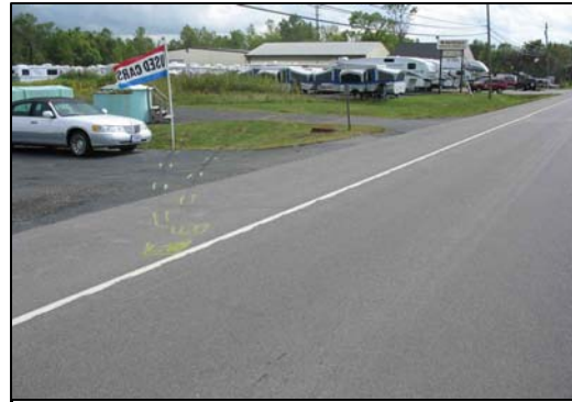
Figure 4 - CW yaw marks leading to the left side road departure.
