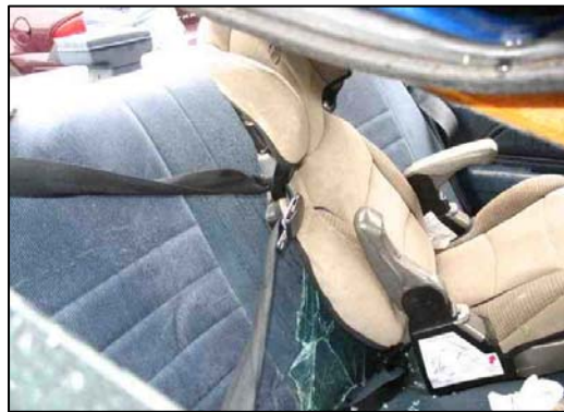
Figure 11 - Right rear belt webbing still engaged in the BPBSS belt path.
