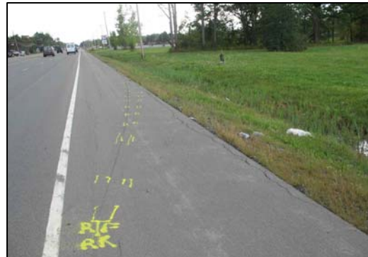
Figure 3 – CCW yaw marks leading to the right side road departure.
