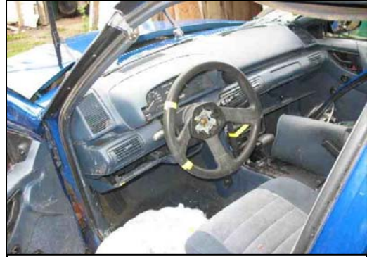
Figure 10 - Contact pattern along the left and center instrument panel.
