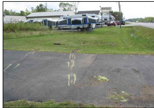
Figure 5 - Deep gouging across asphalt driveway leading to point of impact.
