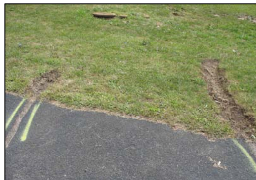
Figure 6 - Trip points leading to overturn.
