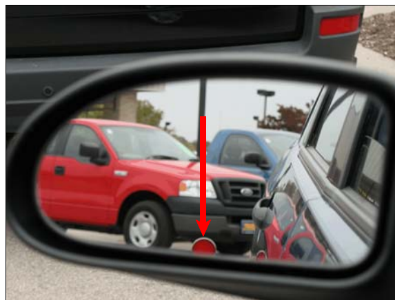
Figure 9: Close view from driver's seat of exemplar Ford Focus through left side view mirror, arrow shows target in location where driver said she could first see it
