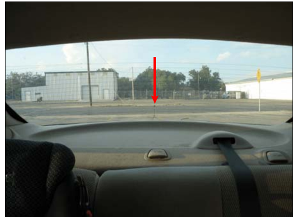
Figure 6: View out of Ford's backlight from driver's seat, arrow shows location of target where driver said she could first see it as she looked over her right shoulder
