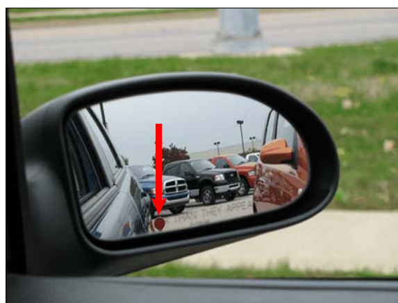
Figure 10: Close view from driver's seat of exemplar Ford Focus through right side view mirror; arrow shows target in location where driver said she could first see it
