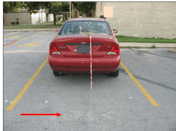
Figure 4: Arrow shows figure representing Ford driver's reported final rest position of pedestrian, dots on Ford's back bumper show area of pedestrian contact, scale in tenths of meter
