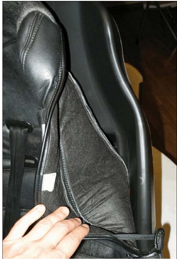
Figure 25: Semicircular stress mark on left side/in-board side of CSS used by Pontiac's second row right passenger
