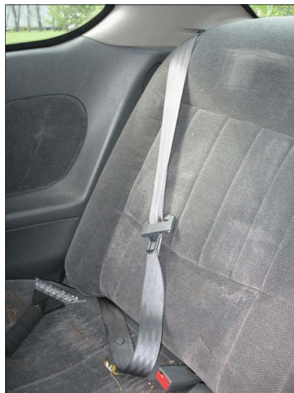
Figure 22: Pontiac’s second row right safety belt showing slight pinching in latch plate but no clear evidence of stress or loading on webbing; Note: wear pattern on seat’s cushion from child seat’s presence
