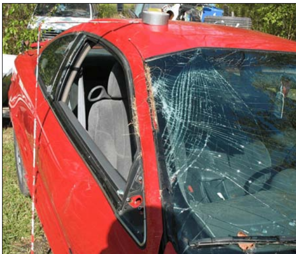
Figure 15: Direct damage to Pontiac’s right side view mirror, A-pillar, windshield’s glazing, roof, and roof side rail; Note: grass in right A-pillar
