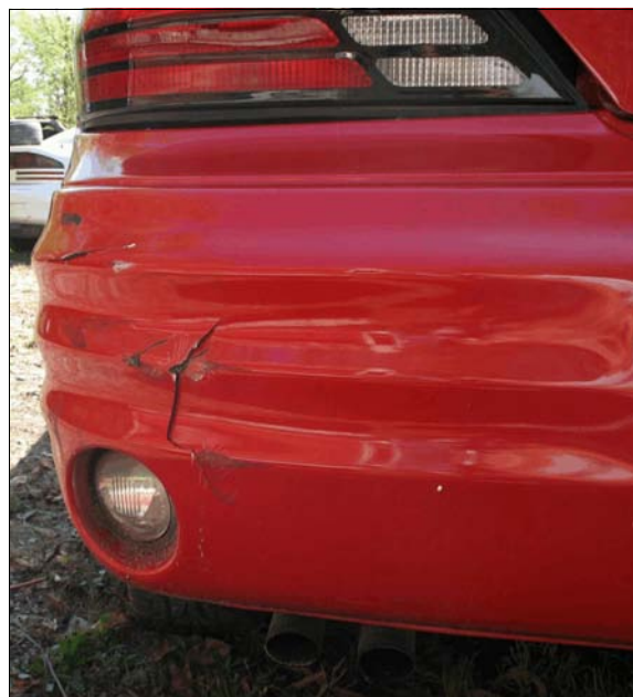
Figure 17: Induced damage to Pontiac’s back left bumper fascia, most likely from impact along left rear side
