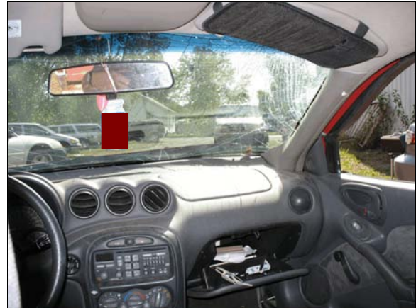
Figure 19: Pontiac's front right seating area showing no evidence of occupant contact to middle and right instrument panel areas and greenhouse area; Note: non-deployed front right air bag
