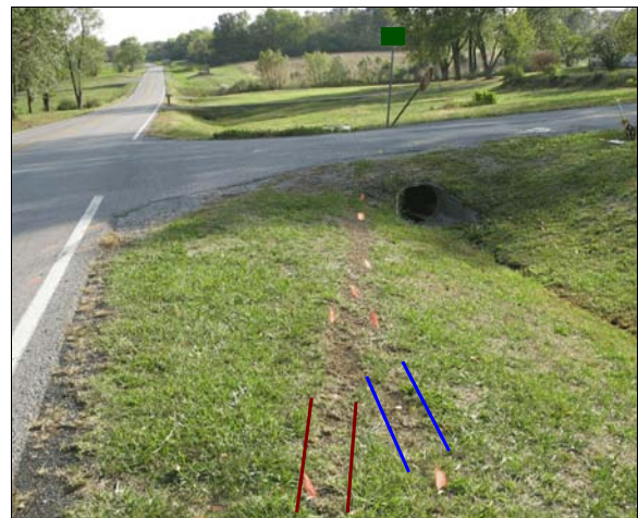
Figure 5: Convergent trajectories of Pontiac’s front tires on south roadside approaching culvert; right lines mark right front tire while left lines mark left front tire
