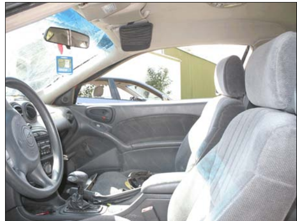
Figure 21: Pontiac's front seating area; intrusions were noted along right roof side rail
