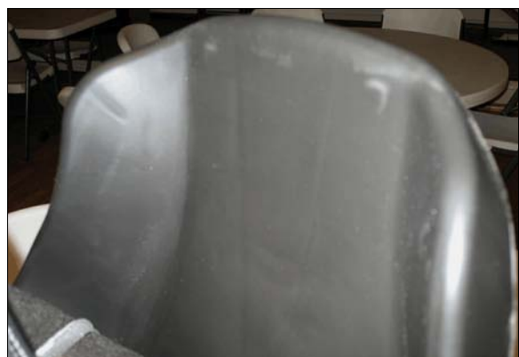
Figure 26: Semicircular stress marks across top of CSS used by Pontiac's second row right passenger
