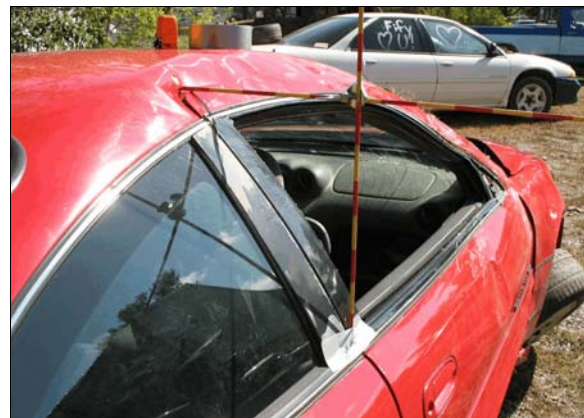
Figure 16: Pontiac’s maximum vertical and lateral crush on right roof rail just above right B-pillar
