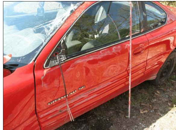
Figure 13: Direct damage to Pontiac’s left side view mirror, left A-pillar and windshield’s glazing, and contact along mid-door level
