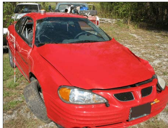
Figure 14: Direct damage to Pontiac’s right front wheel assembly during rollover
