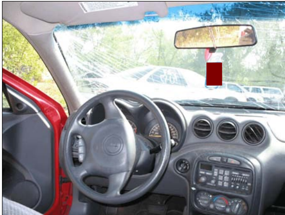
Figure 18: Pontiac's driver seating area showing no evidence of occupant contact to steering wheel, left and middle instrument panels, and greenhouse area; Note: non-deployed driver air bag
