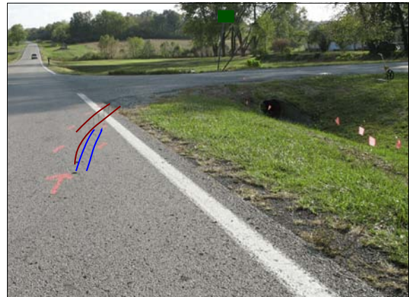
Figure 6: Convergent trajectories of Pontiac's rear tires near south edge line as it travels off road toward impact with culvert; front lines indicate right rear tire, rear lines indicate left rear tire
