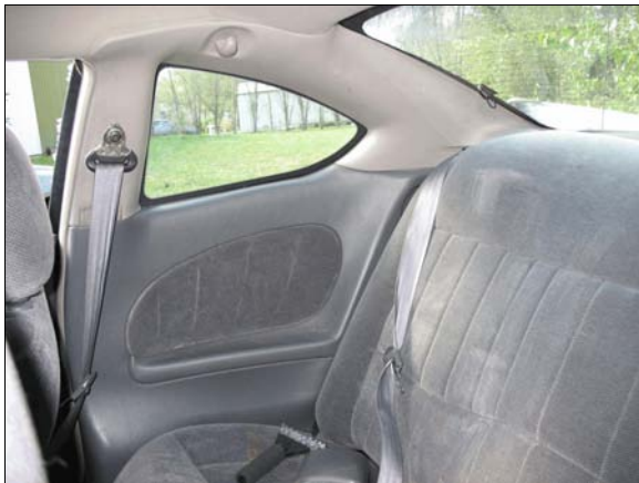
Figure 20: Pontiac's back right passenger seating area showing no evidence of occupant contact
