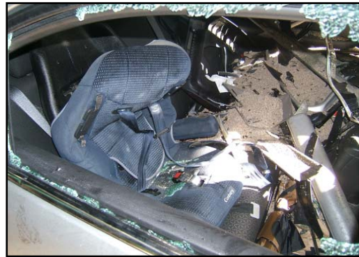
Figure 20. Post crash location of the harness and the harness retainer clips.
