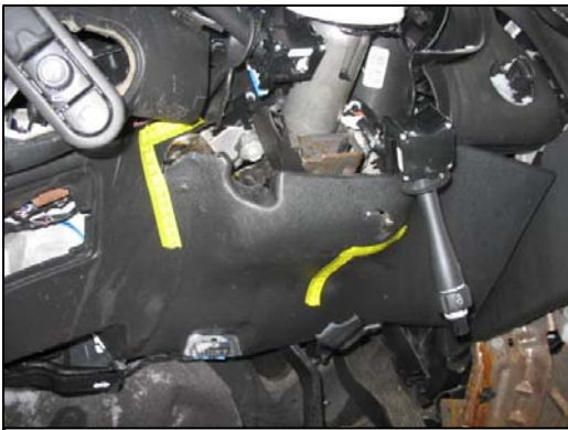
Figure 7 - Knee bolster damage from driver loading.
