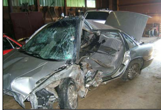
Figure 13 - Frontal and left side damage to the Buick Regal.
