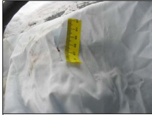
Figure 15 - Small tear in the driver's air bag membrane.
