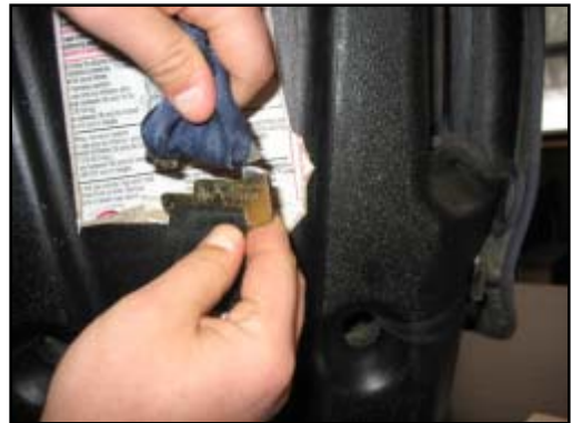
Figure 21. Fractured splitter plate.
