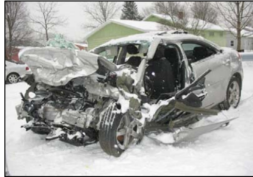
Figure 4 - Damaged frontal plane of Pontiac.
