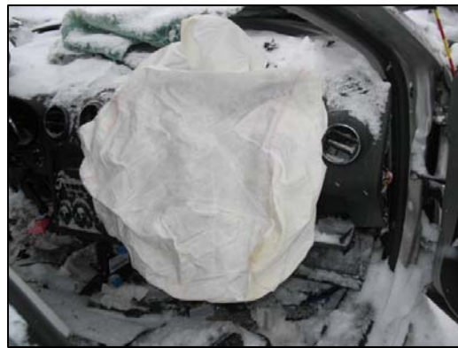
Figure 16 - Deployed front right passenger's air bag.
