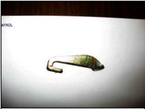
Figure 23. Top aspect of splitter plate. Note the right side attaches to the lower portion of the splitter plate.
