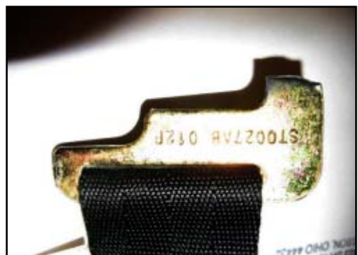
Figure 22. Bottom aspect of the splitter plate. Note the top right aspect is the area of the fracture location.
