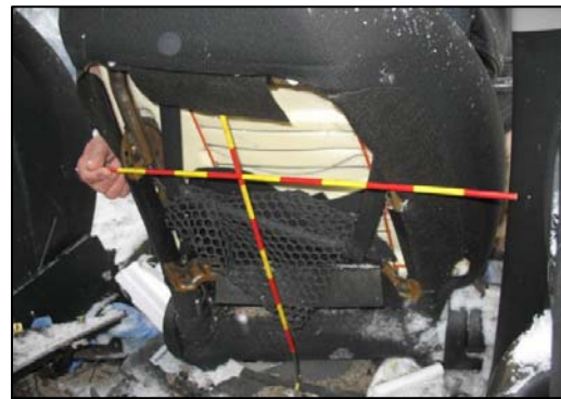
Figure 11 - Damage to front right seat back from right rear passenger loading.
