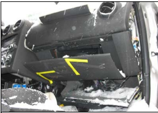
Figure 9 - Damage to glove compartment cover from front right passenger loading.
