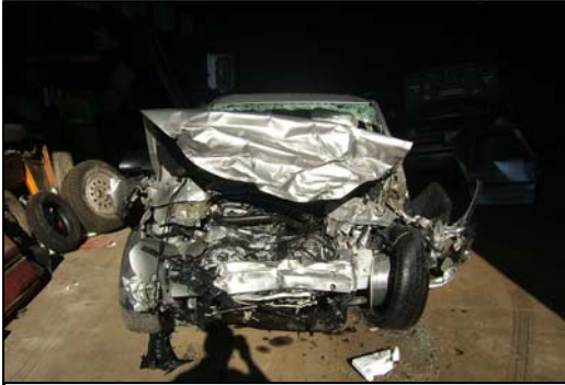
Figure 12 - Frontal damage to the 1992 Buick Regal.
