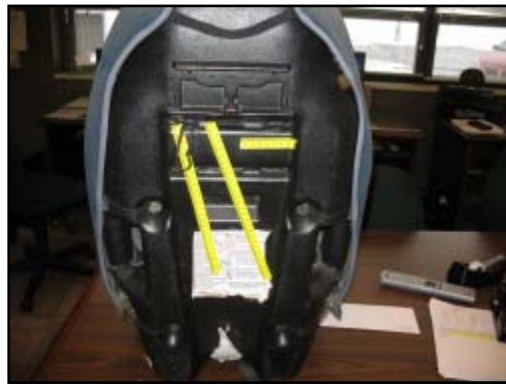
Figure 25. Loading abrasions from the harness straps.
