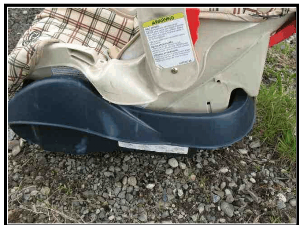
Figure 8. ISS damage (left side of seat in rear-facing orientation).
