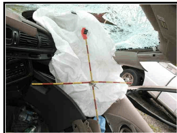
Figure 6. Front right passenger's deployed air bag
