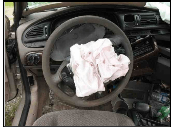
Figure 5. Driver's deployed air bag
