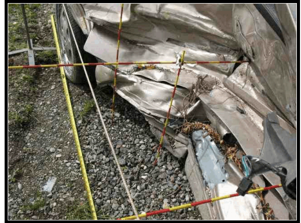
Figure 4. Right side damage, Mercury Mystique
