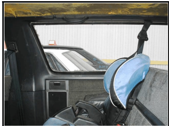
Figure 5. Area of Occupant 3 ejection, right rear window
