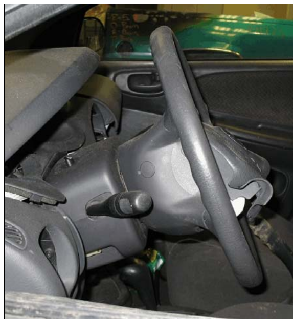
Figure 5: Left side view of the Plymouth's steering wheel showing lack of deformation of the steering wheel rim
