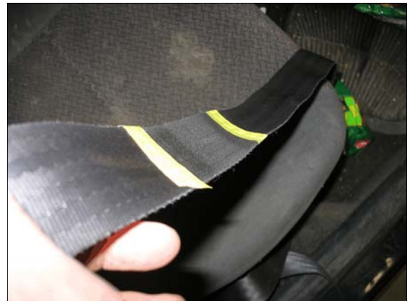
Figure 6: Load mark (between yellow tape) on Plymouth's front right passenger's seat belt
