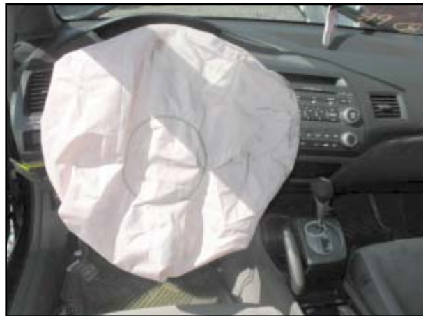
Figure 8. Deployed driver's frontal air bag.
