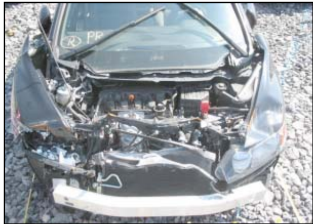
Figure 4. Overhead view of the upper radiator crush.
