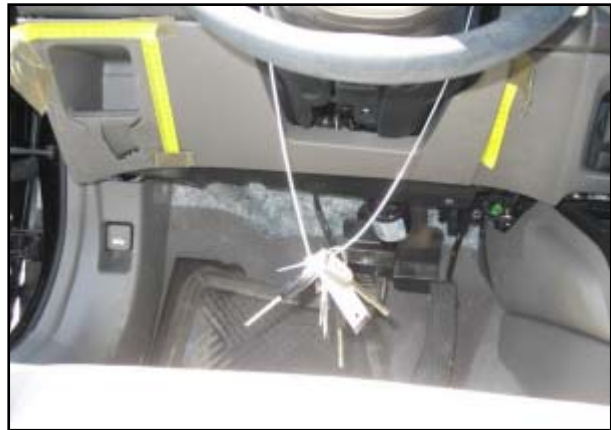
Figure 5. Knee strikes to the left instrument panel.
