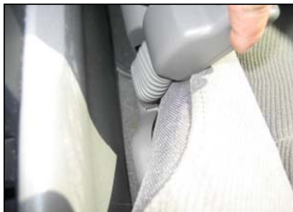
Figure 10. Actuated driver's buckle pretensioner.
