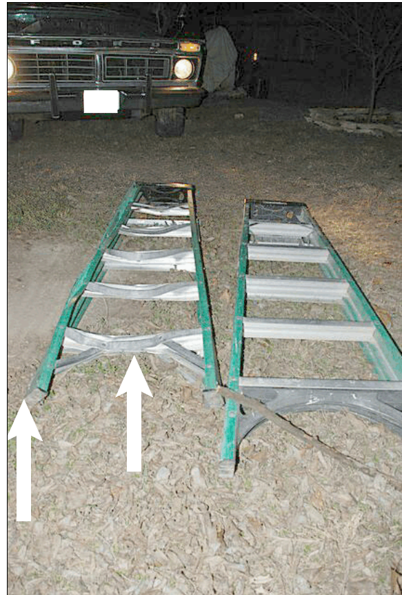
Figure 4: Ladder on left was run over by vehicle's left rear and left front tires; final rest position of Ford in background; left arrow shows left rear tire mark and damage to ladder; right arrow shows damage to ladder from left front tire
