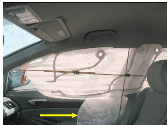
Figure 12: Honda’s deployed right side curtain air bag (front portion); arrow shows deployed front right seat back-mounted side impact air bag
