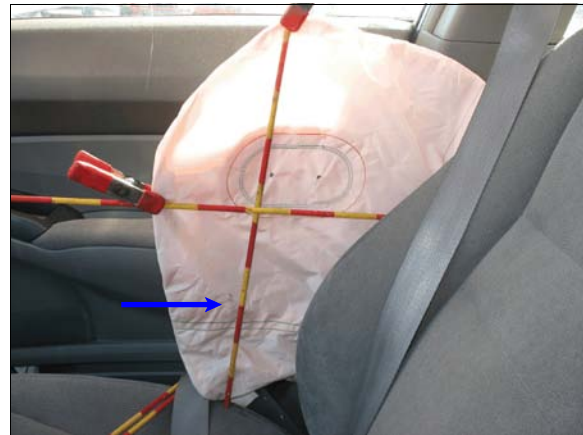
Figure 14: Inboard surface of Honda's front right seat back-mounted air bag; arrow shows location of small dark scuff
