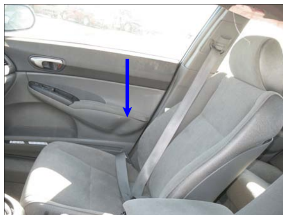
Figure 11: Arrow shows occupant contact dent in armrest of Honda's right front door
