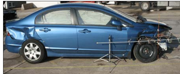
Figure 7: Honda's right side damage from impacts with Mitsubishi—initial impact (event 1) to front, side slap impact (event 2) to rear
