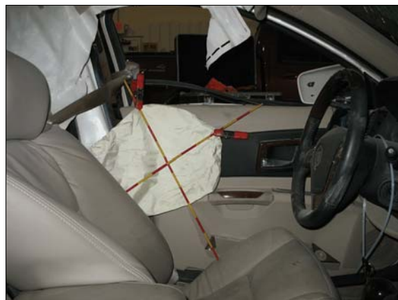
Figure 8: Driver's seat back-mounted side impact air bag
