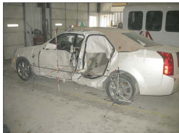
Figure 4: Damage to left side of Cadillac from impact with the Jeep
