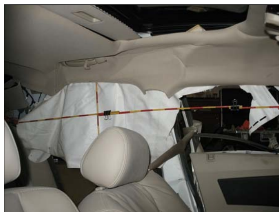
Figure 9: Left side curtain air bag; front portion of air bag cut out by fire department
