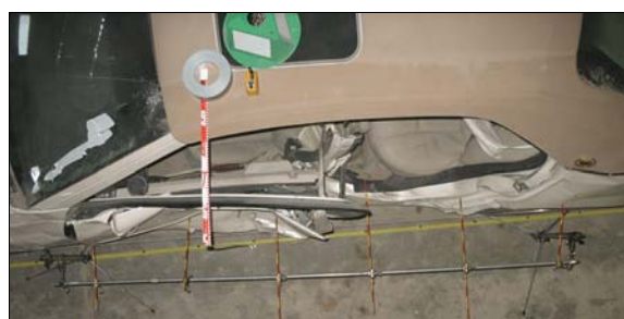
Figure 5: Top view of crush to left side of Cadillac
