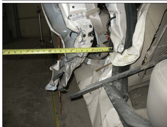
Figure 6: Back to front view of crush to lower portion of the left “B”-pillar
