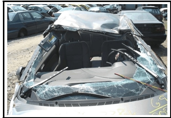
Figure 11. Frontal view showing roof crush sustained during rollover
