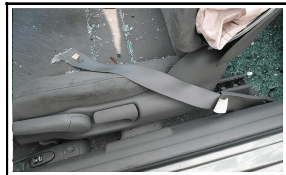
Figure 5. Driver's safety belt webbing was cut during extrication efforts.
