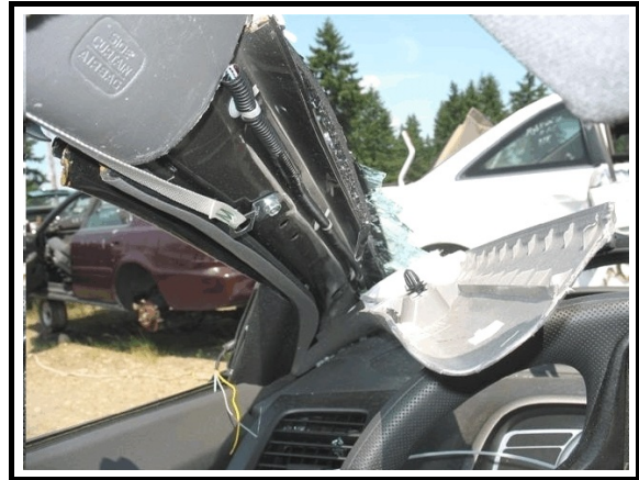
Figure 4. Interior damage, left A-pillar
