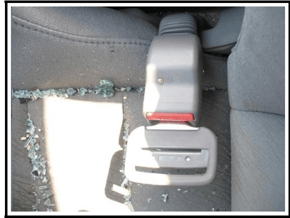
Figure 6. Driver's safety belt latch plate was found in buckled position
