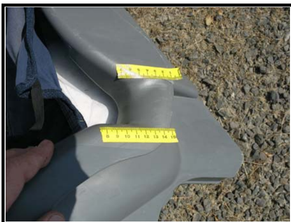
Figure 11. Loading to left lower seat belt guide
