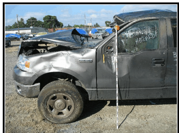
Figure 7. Left side damage from post impact
