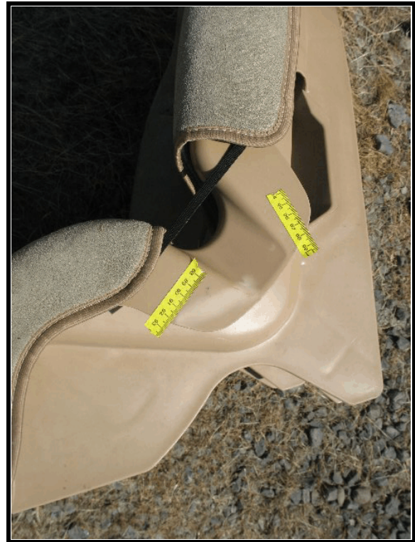
Figure 9. Scuffed plastic loading mark to left lower belt guide
