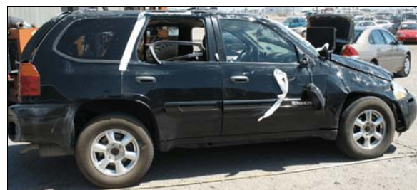
Figure 5: Damage from the rollover on the right side of the GMC; second row left and right passengers ejected through right rear window opening
