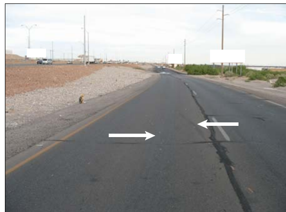
Figure 4: Driver steered left (arrow on left shows right front yaw mark; arrow on right shows right rear yaw mark) and GMC departed north side of roadway
