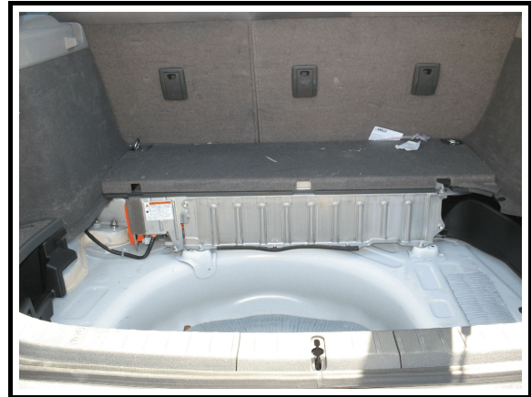
Figure 4. Battery module, located beneath second row seats
