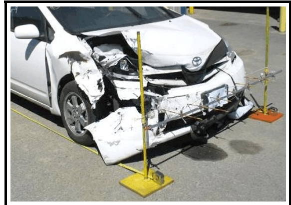
Figure 3. Subject vehicle showing front end crush measurement
