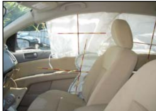
Figure 7. Front right curtain air bag and the seat back mounted side impact air bag.
