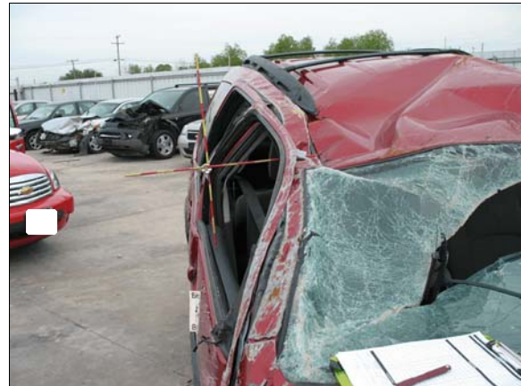
Figure 6: Scale shows the maximum vertical and lateral crush of right roof side rail, each increment in 5 cm (2 in)
