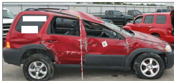
Figure 3: Damage to right side and top of the Mazda from the rollover; vertical scale in tenths of meter
