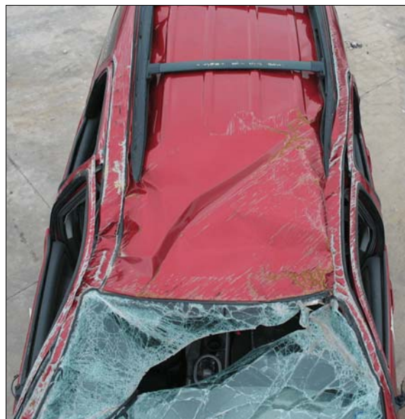
Figure 4: Damage to the top of the Mazda from the rollover, pavement scratches formed in three directions
