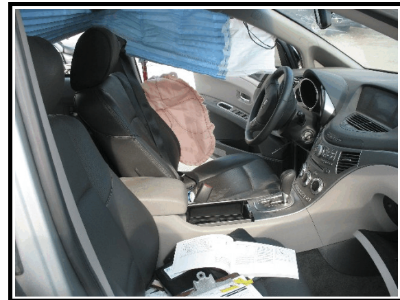
Figure 12. Interior view, side air bags
