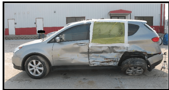
Figure 6. Left side damage, Subaru Tribeca
