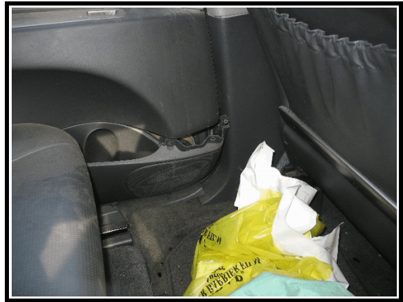
Figure 8. Left lower door intrusion
