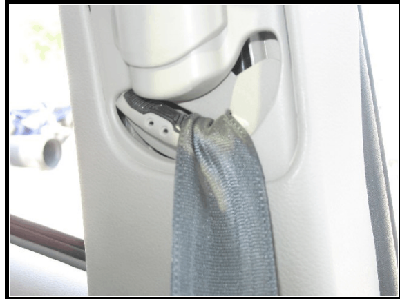
Figure 9. Driver's belt restricted in used position
