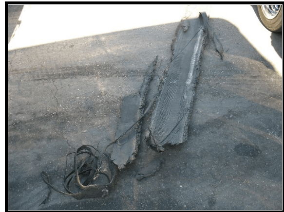
Figure 8. Tread from front axle 1, left tire
