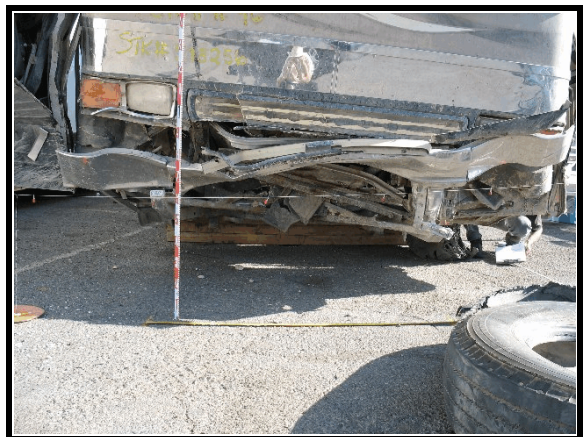
Figure 9. Front bumper damage
