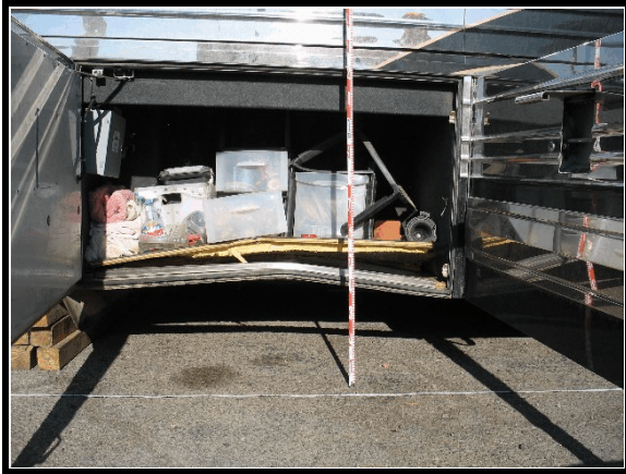
Figure 10. Left side rail/floor vertical crush
