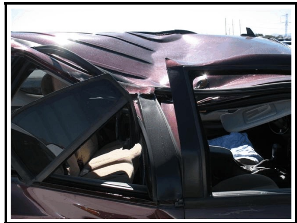
Figure 6. Damage to right roof rail
