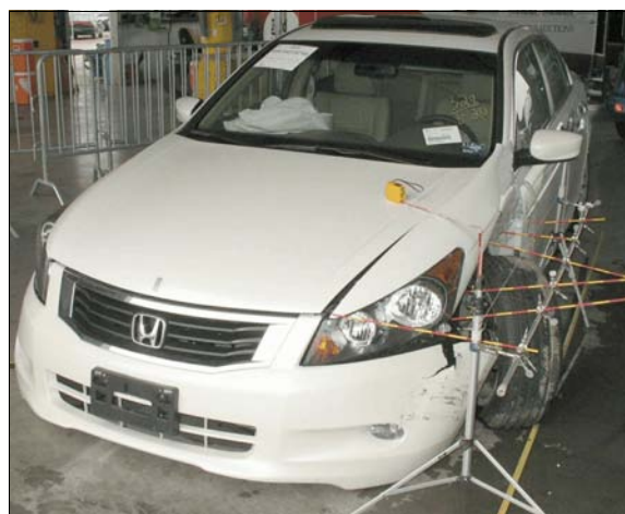
Figure 3: 2008 Honda's left front damage from impact by front of 1991 Honda
