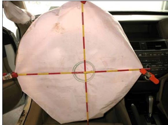
Figure 10: Honda's deployed driver air bag showing only deployment scuffs on bag's surface
