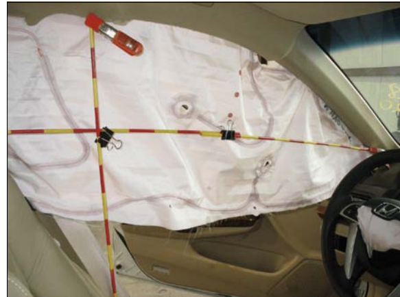
Figure 16: Inboard surface of 2008 Honda's other side inflatable (curtain) air bag showing no apparent occupant contacts along driver's seating portion of bag's surface
