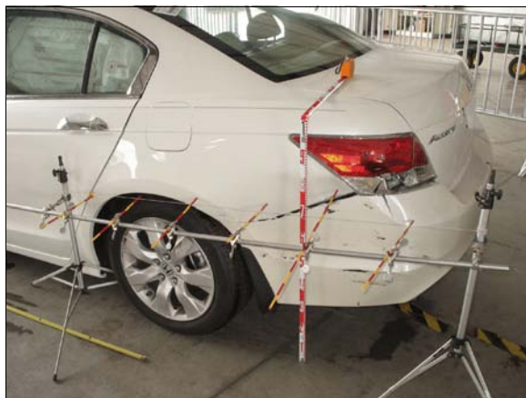
Figure 7: Side slap damage to 2008 Honda’s left rear from impact with right side of 1991 Honda
