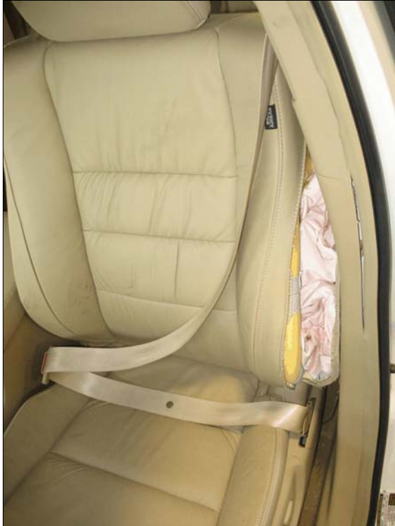
Figure 12: Location of 2008 Honda's deployed driver side impact air bag
