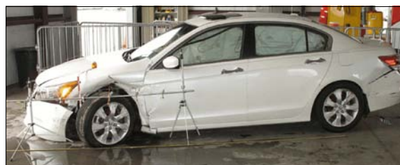
Figure 4: Damage to 2008 Honda's left side from impacts with 1991 Honda; initial impact to left front and subsequent side slap impact to left rear
