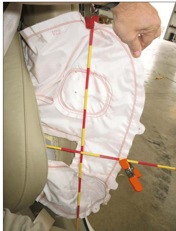
Figure 14: Interior surface of 2008 Honda's deployed driver side impact air bag showing no apparent evidence of occupant contact
