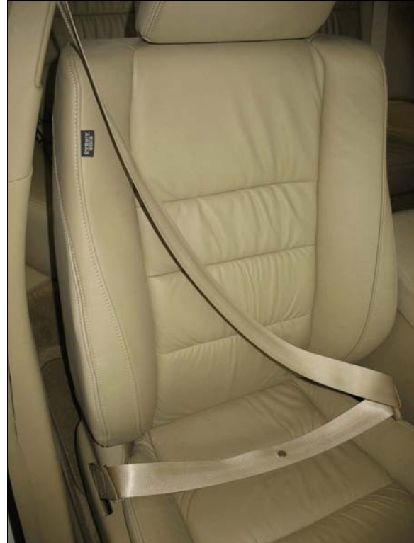
Figure 13: Location of 2008 Honda's non-deployed right front side impact air bag
