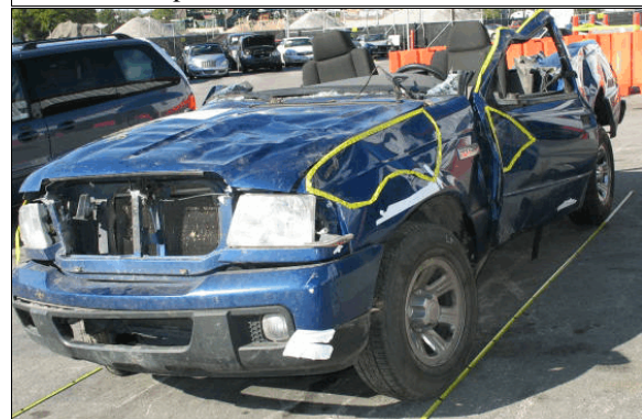
Figure 8: Damage to the Ford's hood and left side from the rollover
