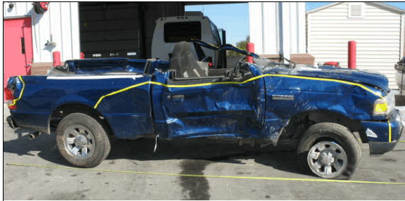
Figure 6: Damage to Ford's right side from the initial touchdown on the north stream embankment during the first quarter turn of the rollover
