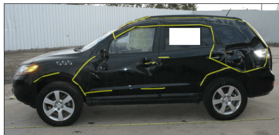
Figure 5: Damage to the Hyundai's left side plane from the rollover (outlined in yellow tape)
