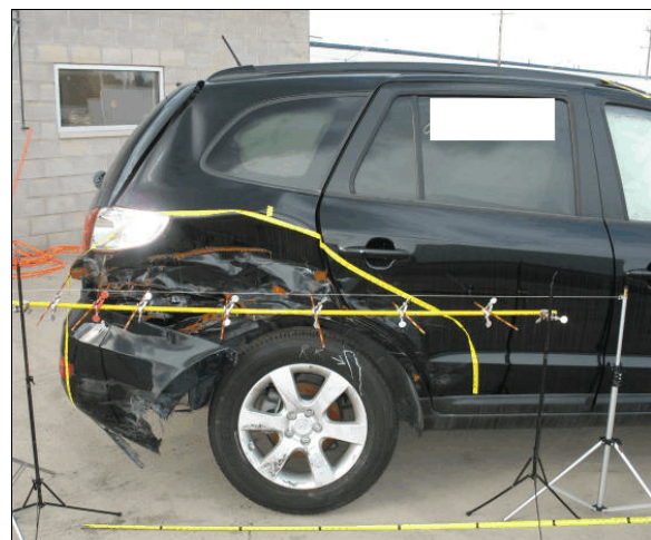
Figure 4: Damage to the right quarter panel, right rear wheel and right rear door from impact with the front of the Jeep
