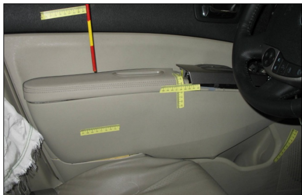
Figure 6: Interior intrusions of the left front door.
