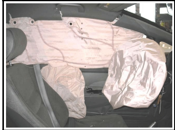
Figure 4. Deployed air bags, subject vehicle
