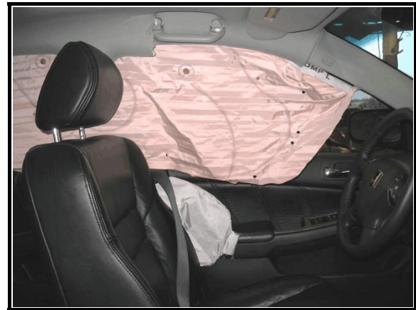
Figure 6. Deployed side impact inflatable curtain air bag
