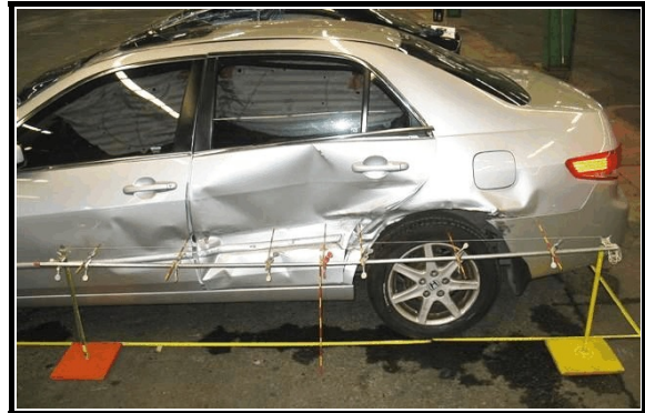
Figure 4. Crush measurement left side
