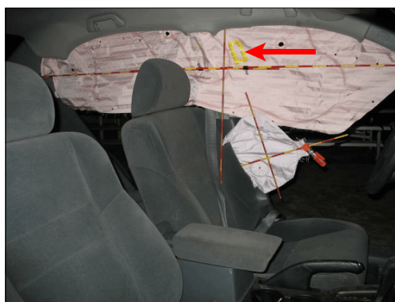
Figure 9: The Honda's deployed left side curtain air bag and seat-back-mounted side impact air bag; arrow shows location of a probable occupant contact scuff mark
