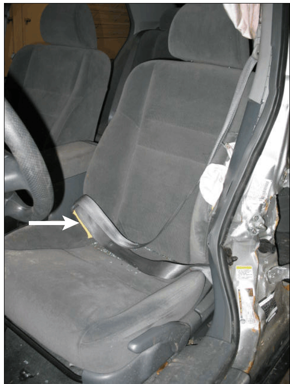
Figure 11: Driver's seat belt; arrow show location of load mark
