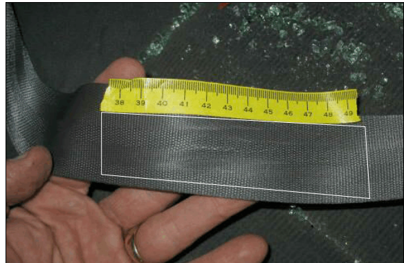
Figure 10: Area of stretching and wrinkling on driver's seat belt, outlined in white
