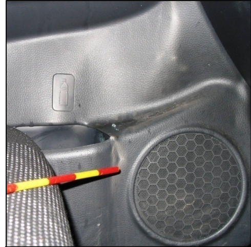
Figure 8: Interior door panel intrusion of the Suzuki.
