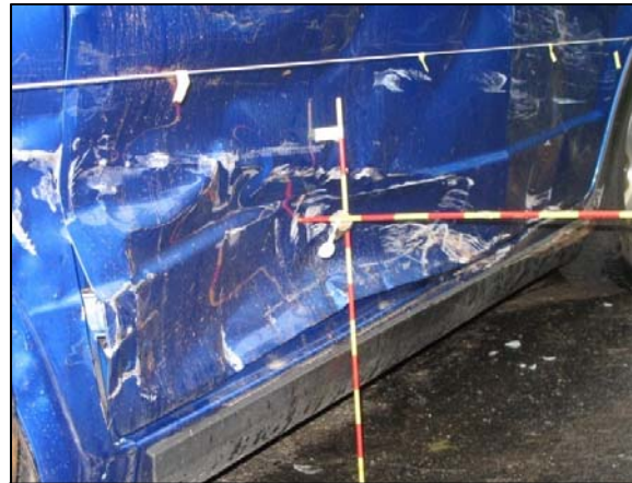
Figure 7: Exterior crush to the left front door of the Suzuki.
