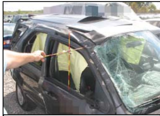
Figure 5. Location of maximum vertical and maximum lateral crush.
