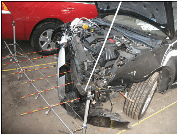
Figure 5: The Mercury’s front crush viewed from left front corner
