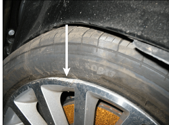
Figure 3: Arrow shows dent and abrasion on right front rim due to curb impact
