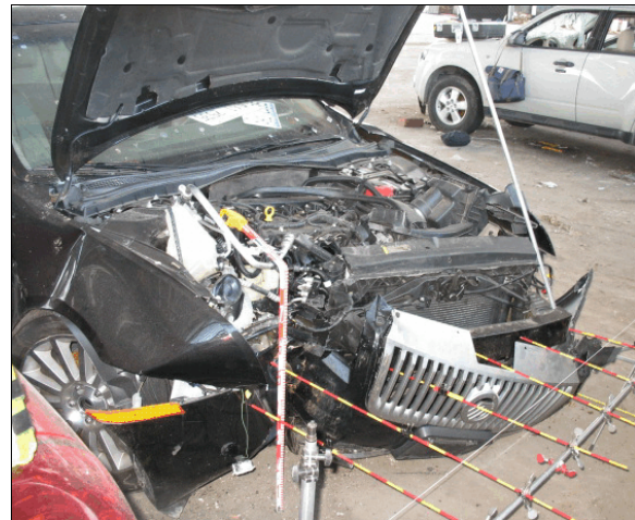
Figure 1: Front damage to the 2008 Mercury Milan Premier from impact with a tree
