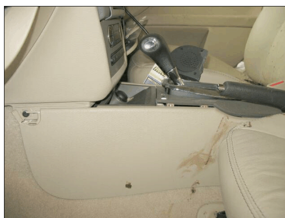
Figure 8: Center console was cracked and displaced to the right
