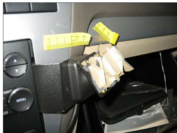
Figure 10: The bent GPS bracket
