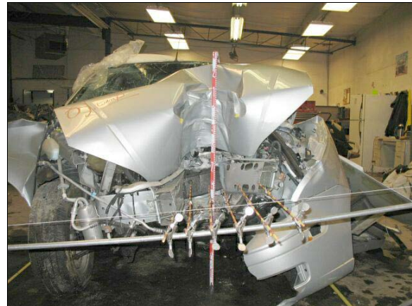
Figure 3: Ford's frontal damage
