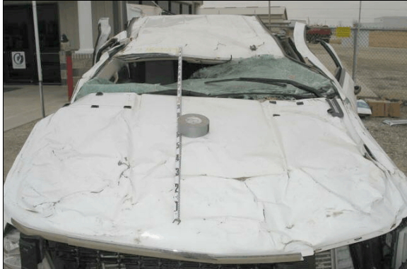
Figure 7: Front view of the top plane damage
