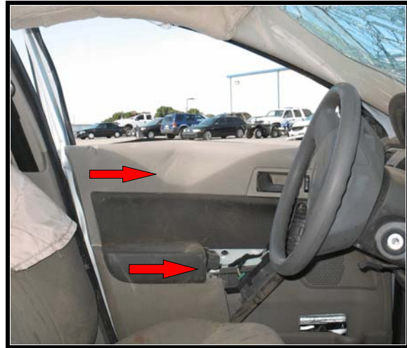
Figure 10. Scratches to door panel and fractured arm rest
