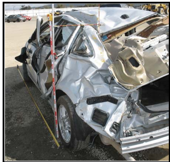
Figure 5. Area of maximum vertical crush
