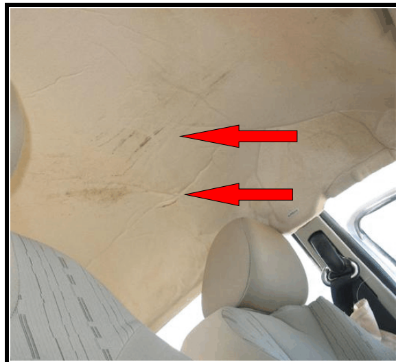
Figure 9. Hair deposit and black marks on roof
