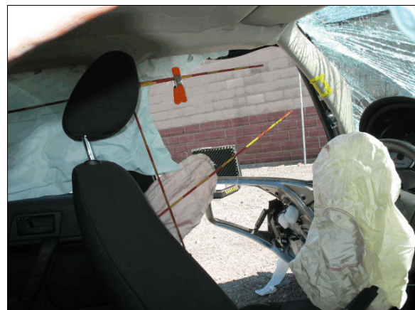
Figure 14: The left side impact curtain air (front portion cut away), seat back mounted side impact air bag and the frontal air bag
