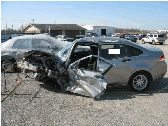
Figure 5: The damage extended down the left side of the Focus breaking off the left front wheel and crushing the left front door
