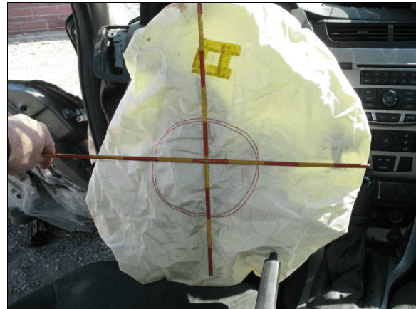
Figure 13: The driver's frontal air bag; yellow tape shows probably occupant contact scuff
