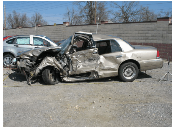
Figure 6: The damage extended down the left side of the Crown Victoria displacing the left front wheel rearward and crushing the left front door
