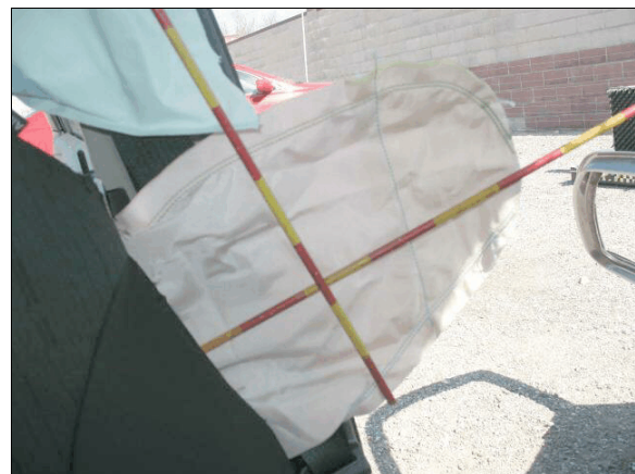
Figure 15: The deployed front left seat back-mounted side impact air bag
