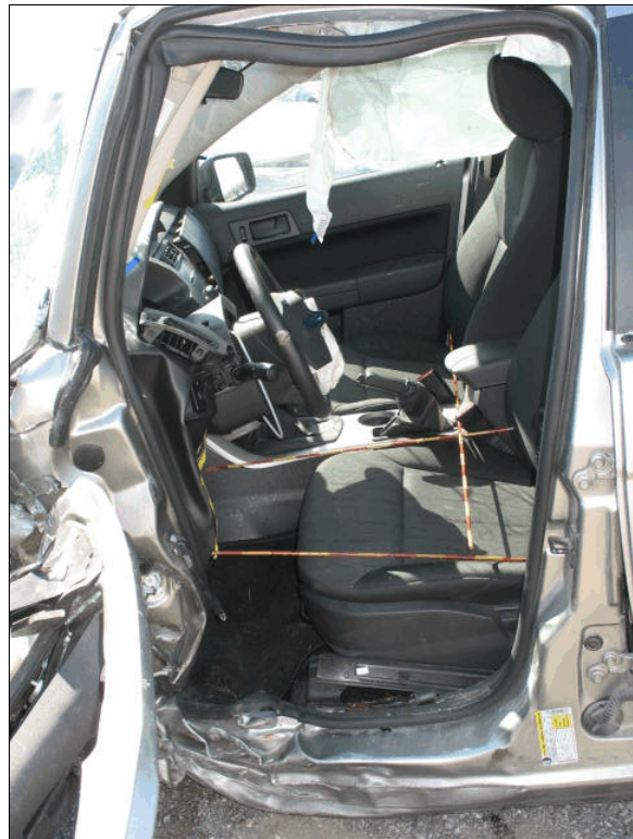
Figure 11: Passenger compartment intrusion
