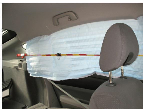
Figure 10: Rear portion of the left IC air bag
