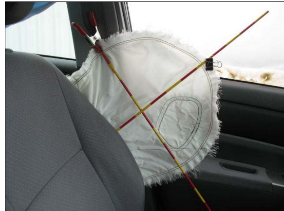
Figure 11: Driver's seat-mounted side impact air bag
