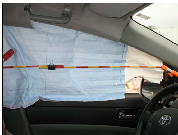
Figure 9: Front portion of the left IC air bag
