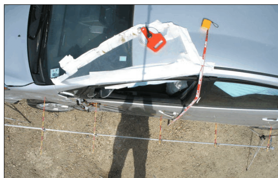
Figure 4: Top view of the Prius’ left side crush
