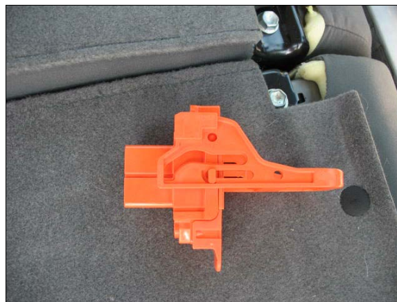
Figure 8: High voltage disconnect plug
