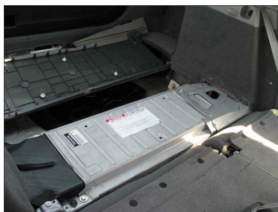
Figure 6: Prius' NiMH propulsion battery case located immediately behind second row seat
