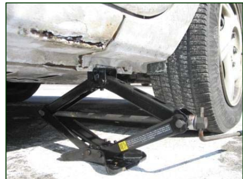
Figure 12. Aft view of the recommended jack position of the exemplar vehicle.
