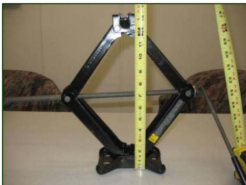
Figure 4. Maximum extension of the exemplar jack.
