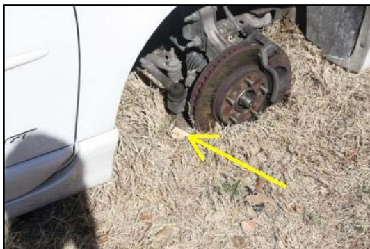
Figure 13. Wood block under the right front brake rotor. (Image provided by the investigating police department.)
