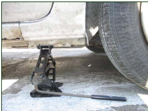
Figure 11. Exemplar vehicle manufacturer’s recommended position of the jack at the right front position.
