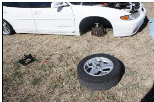
Figure 14. Post-incident status of the OEM scissors jack and the removed right front tire. (Image provided by the investigating police department.)
