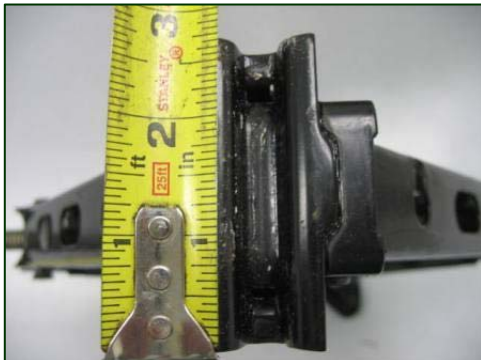
Figure 6. Length of the saddle of the exemplar jack.
