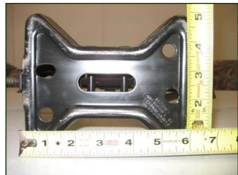
Figure 5. Base dimensions of the exemplar jack.
