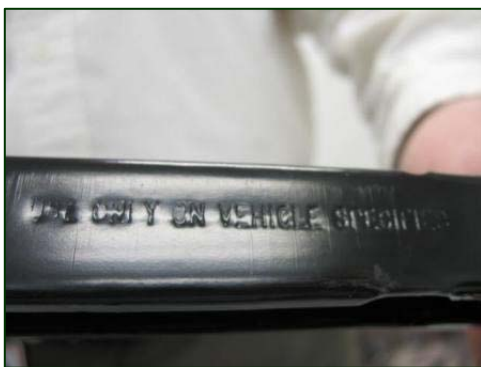
Figure 8. Stamped warning on the exemplar jack.
