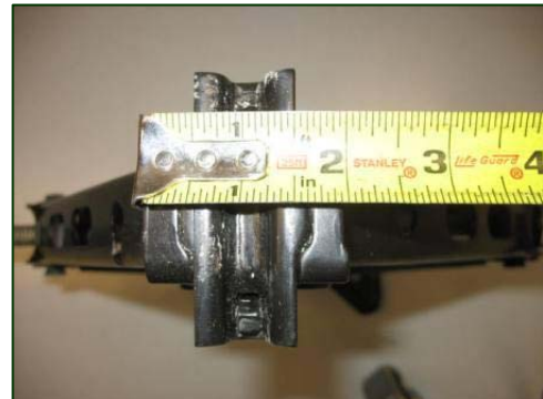
Figure 7. Width of the saddle of the exemplar jack.
