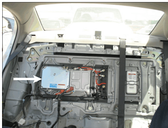
Figure 6: Arrow shows the NiMH propulsion battery box
