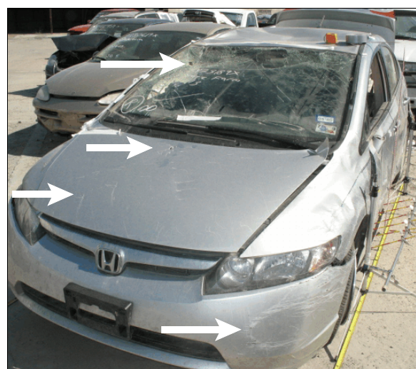
Figure 5: Damage from the rollover on the top and left side planes; arrow at bottom shows damage on the front plane from fence impact (event 1); other arrows show damage on the hood and windshield from the fence that occurred during the rollover (event 4)
