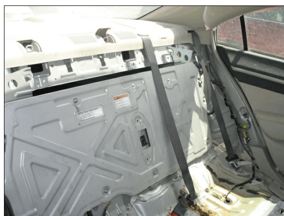
Figure 7: The metal compartment located behind the second row seat back, which contained the NiMH propulsion battery box
