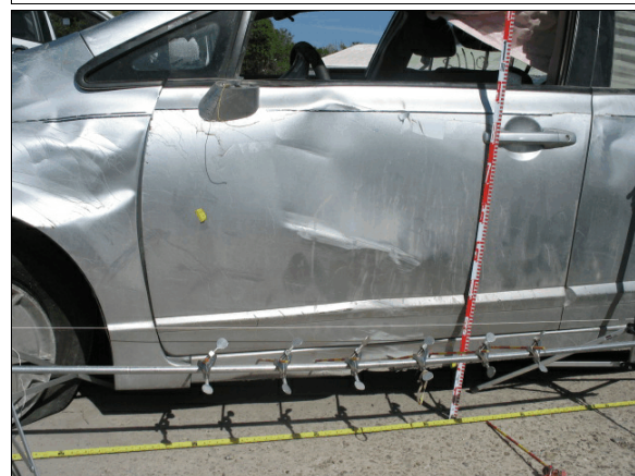
Figure 4: Damage to the left front door from a fence post
