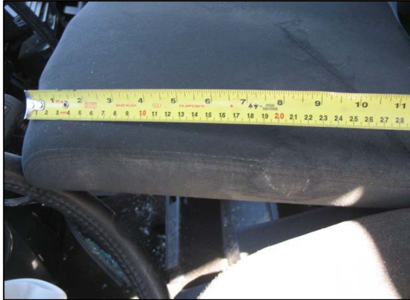
Figure 9: Residual evidence to the center seat cushion from the 11 o'clock vent port.
