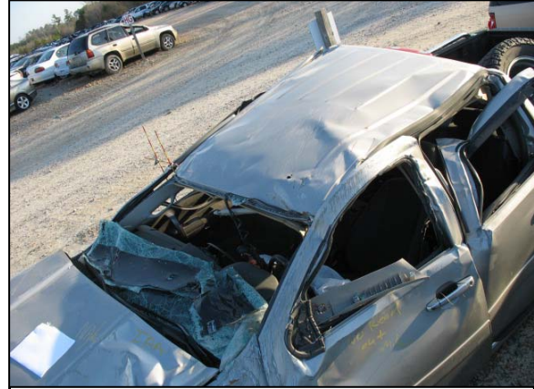
Figure 6: Rollover damage to roof.
