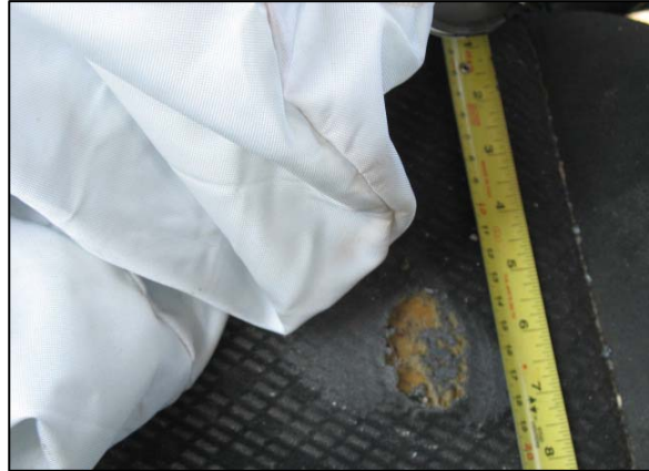
Figure 10: Burn to the driver seat cushion from the 1 o'clock vent port of the driver air bag.
