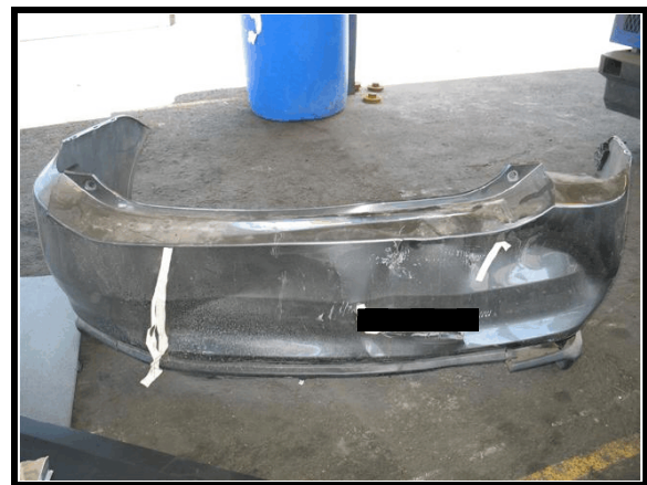
Figure 5. Contact to rear bumper fascia
